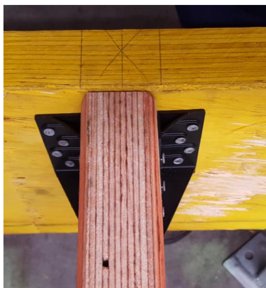
Figure 2: Example of joist hanger tested
