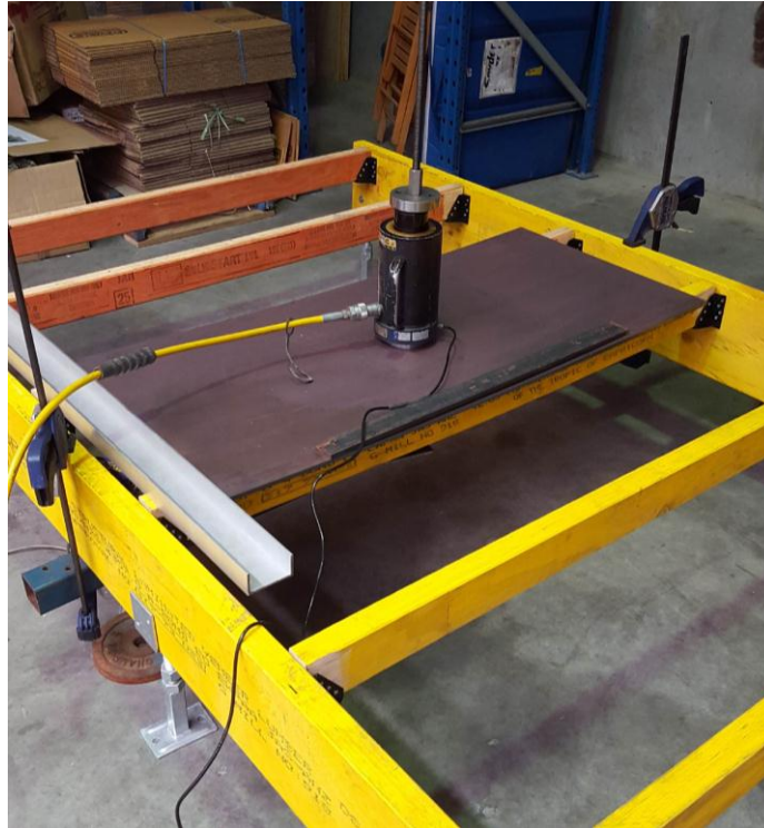
Figure 1: Joist hangers test setup
