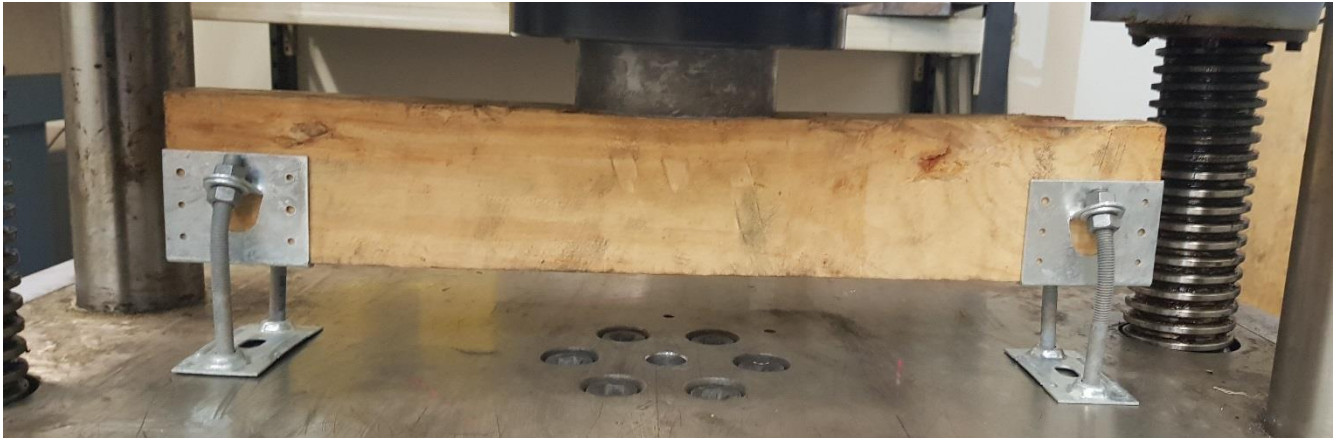
Figure 5: Pair samples after maximum load.
