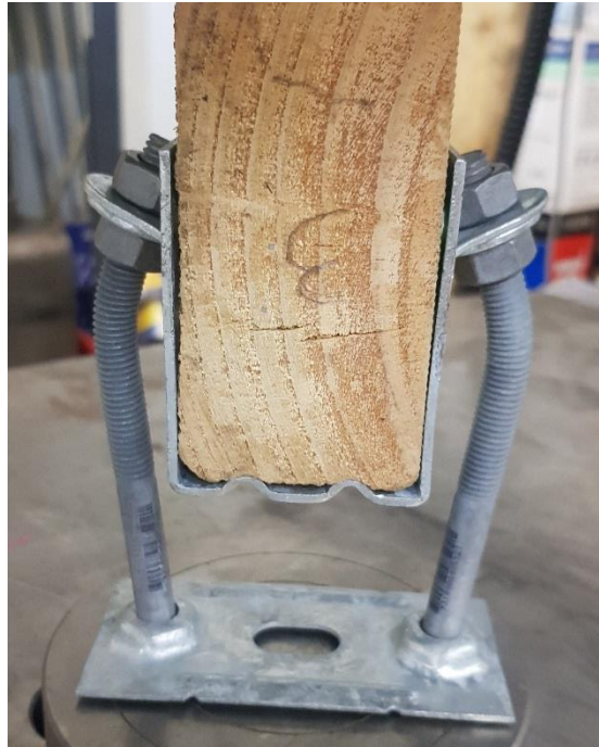
Figure 3: Single sample after maximum load.
