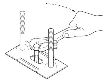
Attach joist Support onto hex bolts and adjust to approx height required. Semi-tighten nuts – this will tighten the whole structure enough to withstand joists being inserted and secured.
