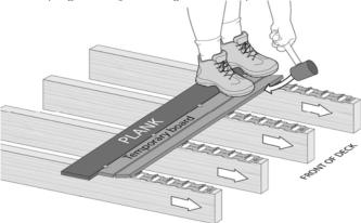
As the leading edge of the board engages with the leading teeth, the trailing edge will move clear of the trailing teeth on the other side of the board, allowing the board to sit flat on the base of the clip. Adjust your foot-pressure to be fully across the board, pushing it fully down on the clip.
