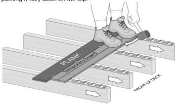
Before using the fixing tool to lock the board into the clip, ensure that the teeth are correctly locating into the board across the following 5-6 joists from the teeth you are about to "lock". Lock the teeth into place at the first joist using the fixing tool. Move along the length of the board repeating this procedure.
